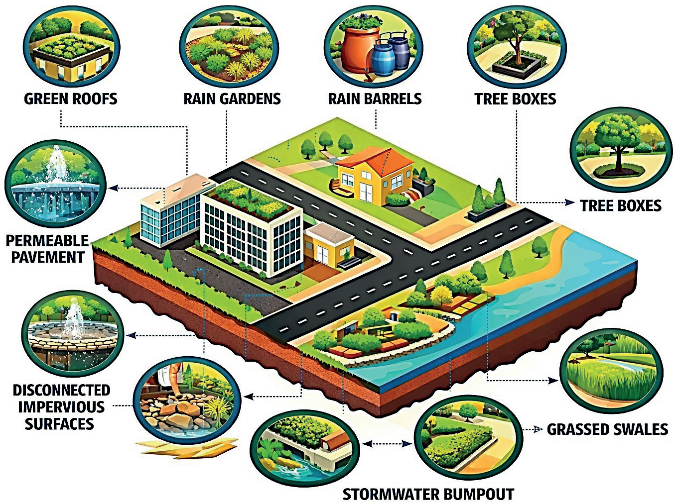
Figure 7: Low Impact Development for Stormwater (Source: TCE)
