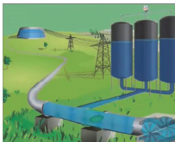
Surge vessel under operation of the pump
